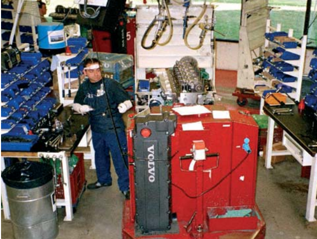
For several years, the National Institute for Working Life has monitored work at Volvo Powertrain in Skövde. During 2002, a reorganization was carried out with which the earlier model with 'docks' for parallel production (left picture) with an assembly worker in each one, was replaced by a serial production system with an assembly line (right picture).
