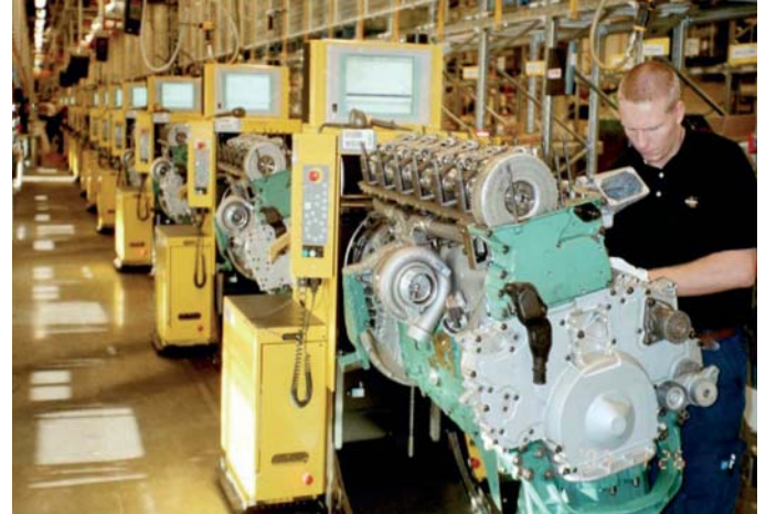
For several years, the National Institute for Working Life has monitored work at Volvo Powertrain in Skövde. During 2002, a reorganization was carried out with which the earlier model with 'docks' for parallel production (left picture) with an assembly worker in each one, was replaced by a serial production system with an assembly line (right picture).
