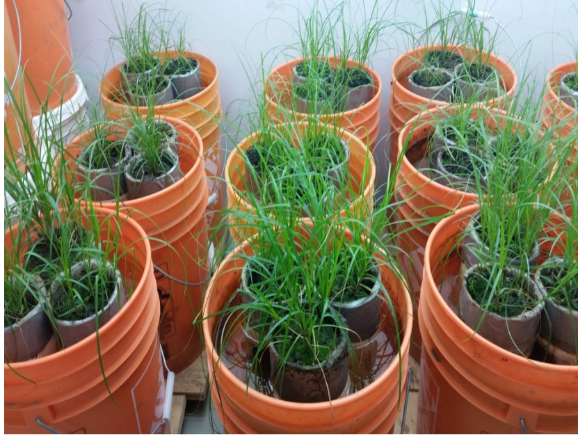
Figure 43: Experimental setup of stationary constructed wetland mesocosm
