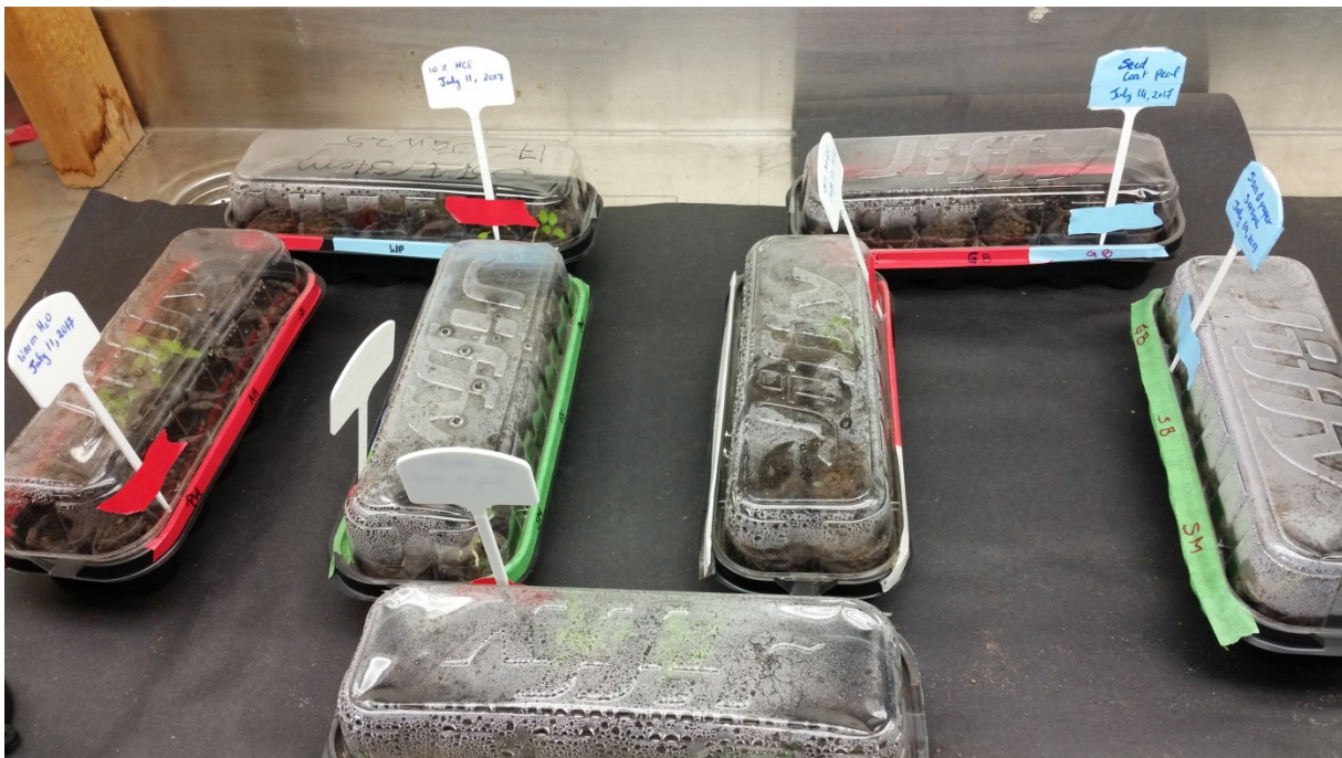
Figure 35: Germination chamber setup for various treatments under light bank
