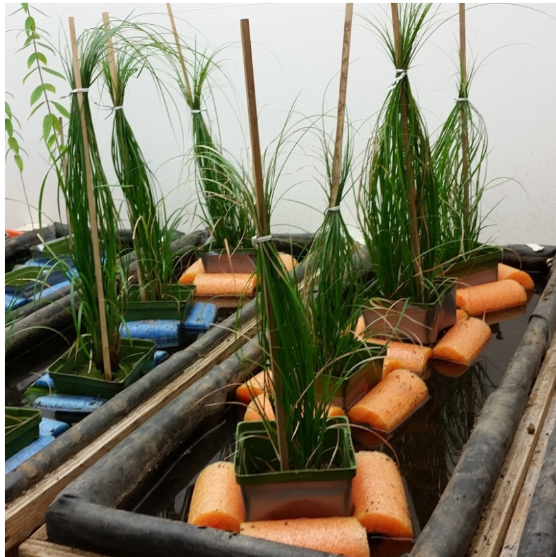
Figure 41: Floating Constructed Wetland Model
