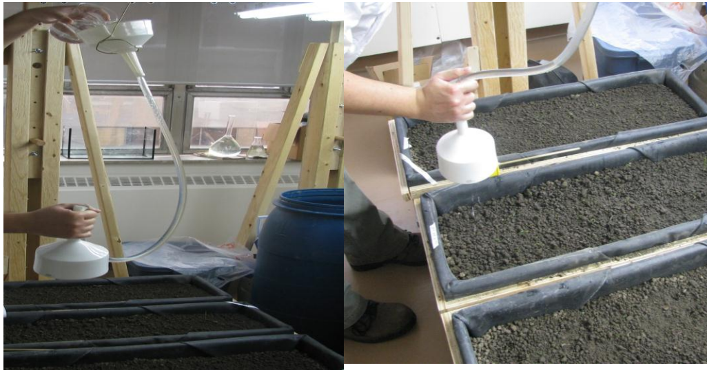
Figure 45: Watering crop troughs via inverted Buchner funnel
