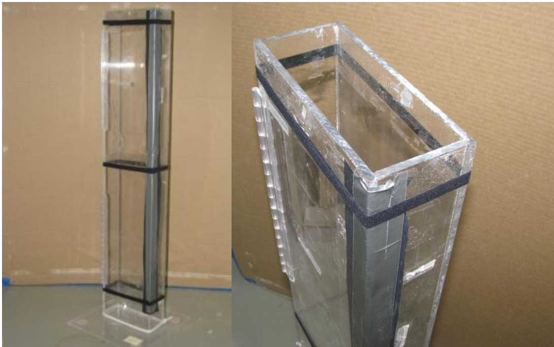
Figure 24: Evan’s Box sealed and ready for filling with soil
