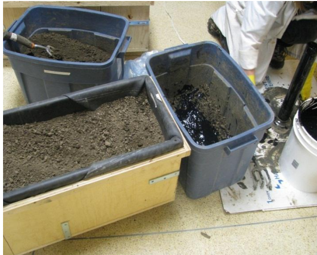
Figure 41: Mixing of biosolids into soil to make treatment soil
