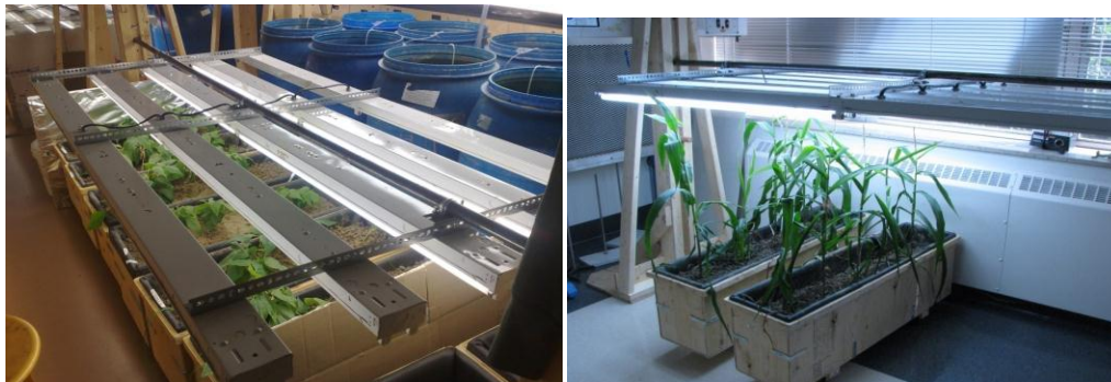
Figure 42: Images of custom made light banks for growing terrestrial plants
