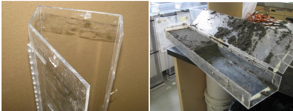
Figure 22: illustration of the hinge design to permit the opening of the chamber
