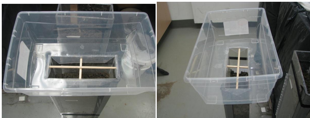
Figure 26: dowels to secure the mating chamber to the top of the Evan's boxes
