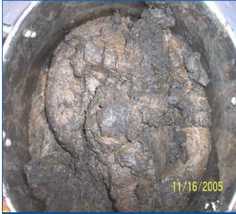
Conventional dewatered biosolids (20%) with a viscosity of > 2,000,000 cp (Lystek 2009)
