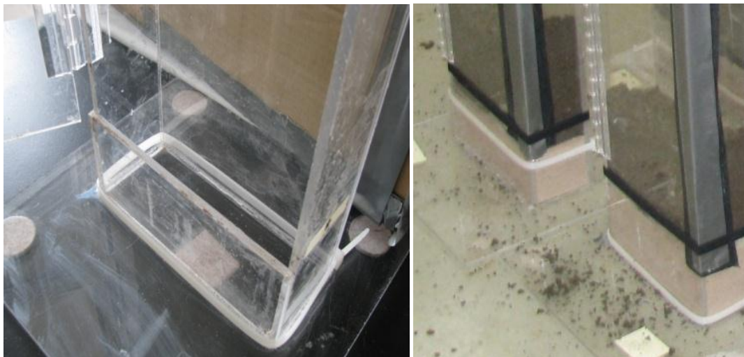
Figure 23: Sand layer at the bottom of the chambers for drainage
