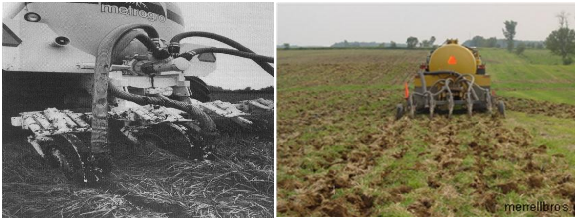
Figure 6: Injection Equipment for Biosolids Application (Source: USEPA 2000b (left), merrellbros.com (right))
