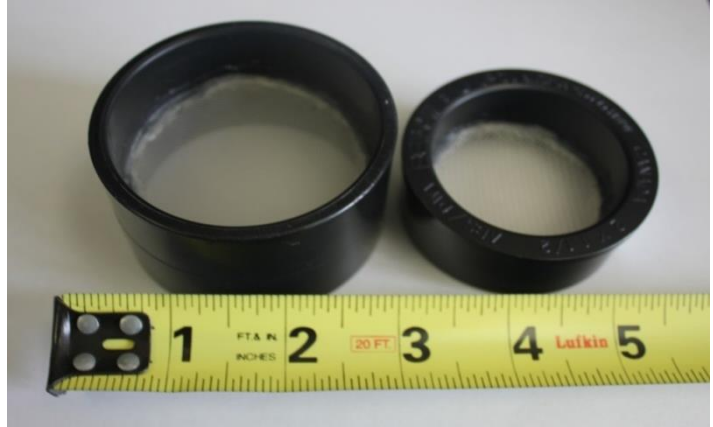
Figure 16 Interlocking screens constructed of PVC piping, Nitex screening, and aquarium glue (M. Raby, 2013)
