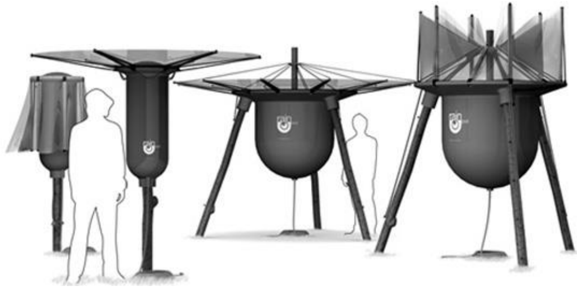
Figure 2: Rainwater harvesting unit with wide rainwater collection area that fold for easy transport.
