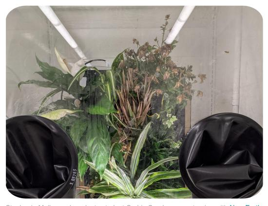
Stephanie Melles and graduate student Corbin Sparks are partnering with <u>New Earth Solutions</u> to study the <u>hydroponic green wall</u> and its ability to remove airborne volatile organic compounds, as well as the microbial system in the root system of the unit.
