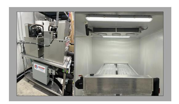
As part of the Jet Ice Research Project, last month miniature ice rinks were installed in the Urban Water Experimental Lab. This month, postdoctoral researcher Ryan Hutchins is working with Accent Refrigeration to set up the equipment and regulate the conditions inside of the cooling chamber. The temperature and humidity in the chamber need to be regulated for ideal ice making conditions.
