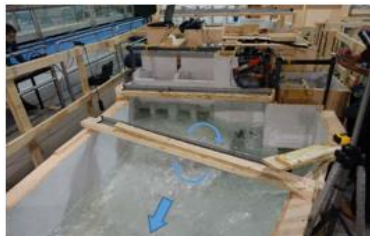
Energy Dissipation at the Stilling Basin
